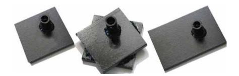
These TLC Tile Breakers easily connect to TLC rods or adapters. Only steel cleaning rods, like the TLC ProKleen Rods, should be used. Use the Small Tile Breaker for 8" x 8" or 7" x 7" flues. For 12" x 12" and larger tiles, use the Large Tile Breaker. The Double Tile Breaker is for 11" x 11" or 8" x 12" flues.
