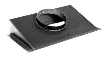
The Round Insert Boots are made with 11 gauge, carbon steel and provide a 20° angle for Ventinox Liner adjustment. Attach the insert to liner with bolts, or by tapping and screwing. The inside base dimensions for this product are  $8 \frac{1}{2}$ " x 16", outside base dimensions are  $10 \frac{1}{4}$ " x 18", with boot height of 4 %".
