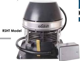
The RSHT Chimney Fan is for use with wood, pellet, or coal applications where flue gas temperatures do not exceed 1400° F for intermittent operation, and 1000° F for continuous operations.
