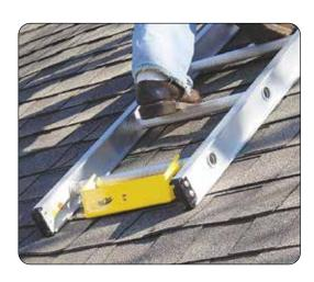
Roof Boots can be used on a 7/12 or greater pitch asphalt or shingled roof providing easy, and safe roof access for a ladder or PiViT Ladder Tool. Roof Boots are easily secured (instructions included), and can provide security with the PiViT Ladder Tool up to 20/12 roof pitches.
