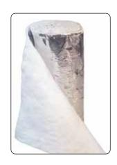
Superwool Plus Insulation Blanket is a nonceramic, foil-faced, insulation wrap with thick, 3 mil. aluminum facing. It's used as an insulator for stainless steel liners in masonry and wood burning chimneys usually taking two wraps of 1/4" or one wrap of  $\frac{1}{2}$ ". This product has no UL Listing.
