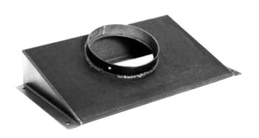
The Round Insert Boots are made with 11 gauge, carbon steel and provide a 20° angle for Ventinox Liner adjustment. Attach the insert to liner with bolts, or by tapping and screwing. The inside base dimensions for this product are  $8 \frac{1}{2}$ " x 16", outside base dimensions are  $10 \frac{1}{4}$ " x 18", with boot height of 4 %".
