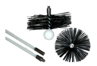
This Pellet/Dryer Vent Brush features quality, nylon bristles, and a guide ball to help prevent snagging. It screws onto Pellet Rods, and is stocked in 3" and 4" diameters. The flexible 4' Pellet/Dryer Vent Rods have a threaded male and female end  $(\frac{1}{4}" - 20 \text{ thread})$ . These are an economical choice for cleaning pellet appliance flues and dryer vent flues, and are for hand brushing only.
