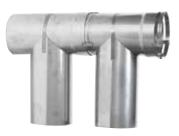
The Double Take-Off Swivel Tee is made with 24 gauge, 316 stainless steel and designed with two take-offs, giving it the capability to spin 360°. This tee features a standard, 2" between take-offs, and comes with an "EZ" band connection.
