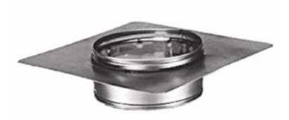
These ICP Masonry Adapters are used when installing the StormShield, Vacu-Stack, or WeatherShield Chimney Caps on a masonry flue. The adapter slides into the flue and secures with a tightening bar in the corners - seal the plate to the flue tile with high-temperature silicone sealant.
