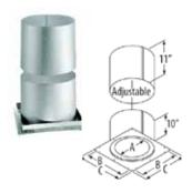
The Firestop Radiation Shield is required for ceiling/floor penetrations when a ceiling support is not used, but is not required for passing through a roof. This shield fits on the ceiling side of the installation and adjusts in height.
