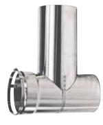
These SmartFlex Two Part Tees are available in 316 or 304 stainless steel, and for use with flex liner (316), or rigid pipe and OD liner (304). The "EZ" band clamp ensures these tees maintain mechanical integrity in extreme heat conditions.
