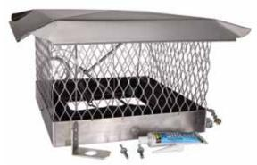
The Energy Top Plus damper combines the efficiency of the Energy Top with the added protection of a stainless steel cap. This damper seals out rain, snow, and sleet while sealing in "paid" heat and air conditioning, but also provides added animal and debris control. The Energy Top Plus does not require a fire safety device, is made of the same material as the Energy Top allowing for easy operation, and comes completely assembled and ready
