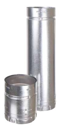
DuraVent Type B Gas Vent Pipe features the DuraLock connecting system, and can be used as a connector, or a standalone vent pipe. This pipe is for use with natural gas fireplaces, gas-fired category I furnaces, boilers, water heaters, and wall or space heating appliances. The recessed, inner wall is .012" aluminum while the outer wall is .018" galvanized and adds 5/8" in wall thickness.
