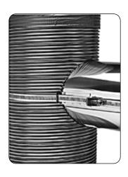
Because of its unique, continuous welded seam, Ventinox VFT Liner is one of the few liner systems in the world that offers the ability to install these Universal Take-Offs directly to the body of the liner. When you drill into Ventinox Liner with a hole saw, we recommend in reverse, it provides a clean cut with no unraveling, allowing the Universal Take-Off to act as a tee snout. The liner must be a minimum of 1" larger
