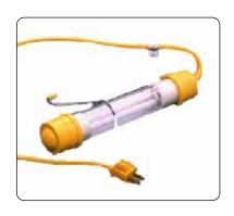
The Stubby Work Light features a high-intensity, 13-watt fluorescent bulb that packs the equivalent light output of a 75-watt bulb It is 10 1/8" long, 10 times more impact resistant than a standard flashlight, and includes a 25' cord with switch and in-line ballast. The Mag Mounts (sold separately) clamp around the Stubby Light and magnetically hold it to a damper frame or metal surface. This product is also available with tool tap option, and replacement bulbs.
