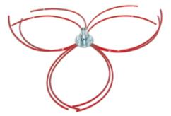
The Stinger Whip set is designed for removing moderate, third-degree creosote build-up. This whip set comes with ButtonLok rod fitting, and should be used with ButtonLok Poly Rods, making removal quick and easy. A 1/2" drill with clutch and drill adapter are recommended when using this product. The Stinger Whip Set is great for quick cleanings, and features ButtonLok Female connectors.
