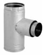
The Increaser Adapter Tee & Cleanout Tee Cap attaches directly to an appliance as an adapter, converting 3" appliance exhausts to 4" PelletVent Pro vent pipe. They are used for 90° offsets, and incorporate a removable, twist-lock Cleanout Tee Cap.
